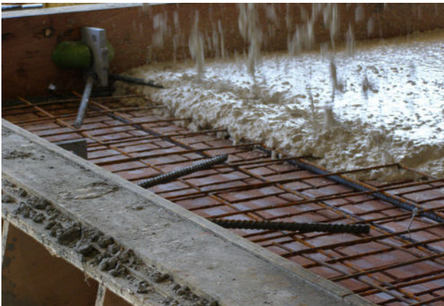
Photo 1 Fabrication of Precast Panel with Thin Brick
