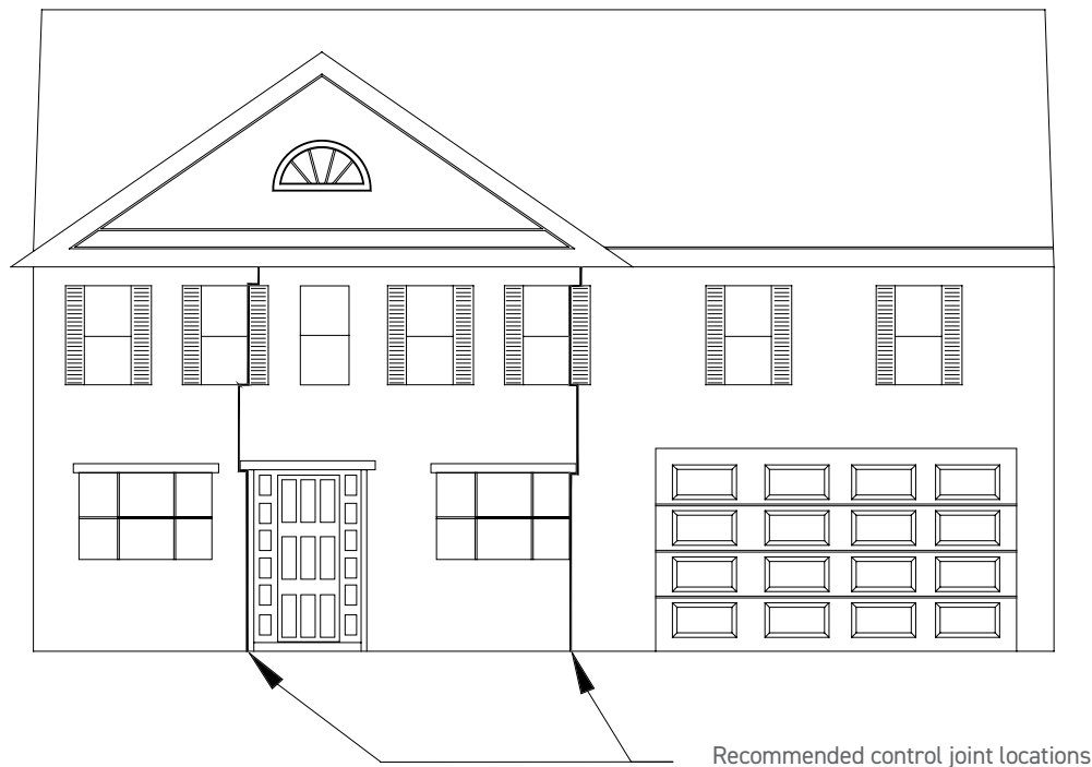
Figure 2 - Example of Residential Control Joint Placement
