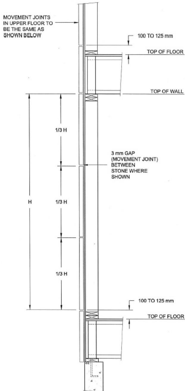
Figure A-3. Required movement joints in applications for the product
